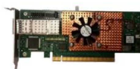
Figure 2: BXIv2 NIC standard PCIe card
